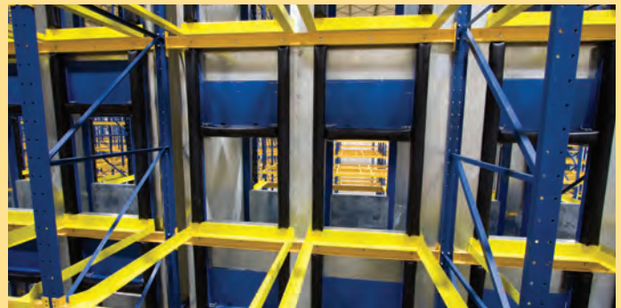
The QFR Zone racking system allows for improved airflow, leading to more efficient freezing.
