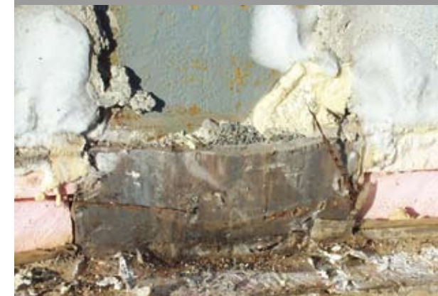
When oak blocks absorb moisture and freeze, they can swell and cause major damage to a warehouse.
